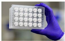
Agilent polyethylene filter microplates can be used in a multitude of high-throughput filtration applications. These filters perform well in protocols where sample debris removal without clogging is needed. Polyethylene membrane filters have excellent chemical compatibility and resistance and can withstand gamma irradiation sterilization. These plates can be used in coarse fractionation and sample preparation for flow cytometry to reduce cell aggregates and clogs.
