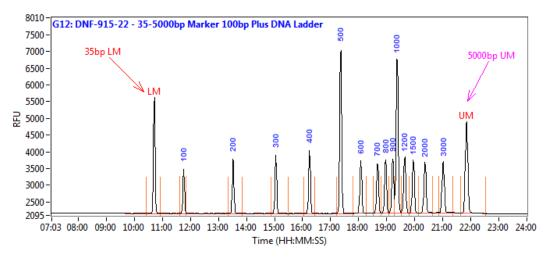
Representative 100 bp Plus DNA Ladder result co-injected with 35 bp lower marker and 5,000 bp upper marker, using the Fragment Analyzer system with the dsDNA 915 Reagent kit. Method: DNF-915-22 ("ultrashort" array). RFU values may differ between instruments.
