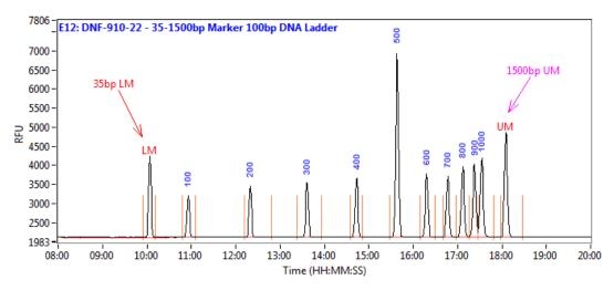
Representative 100 bp DNA Ladder result double injected with 35 bp lower marker and 1,500 bp upper marker, using the Fragment Analyzer system with the dsDNA 910 Reagent Kit. Method: DNF-910-22 ("ultra-short" array). RFU values may differ between instruments.
