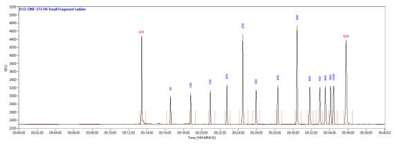
Representative HS Small Fragment DNA Ladder result using the Fragment Analyzer system with the DNF-477 HS Small Fragment kit. The peaks are annotated by size (bp). Method: DNF-477-33 (short capillary array). RFU values may differ between instruments.
