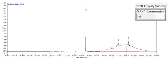
Example mouse kidney ribo-depleted RNA sample result using the Fragment Analyzer system with the DNF-472 HS RNA kit (15 nt). Method: DNF-472M33 (ribo-depleted mRNA analysis method, Capillary Array Short). Peaks annotated by size (nt). The **mRNA Property Summary** is displayed for each sample in the ProSize data analysis software, reporting %rRNA Contamination (% of ribosomal RNA in the total concentration). RFU values may differ between instruments.
