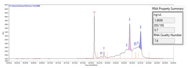
Example Universal Human Reference total RNA sample result using the Fragment Analyzer system with the DNF-472 HS RNA kit (15 nt). Method: DNF-472T33 (Total RNA analysis method, Capillary Array Short). Peaks annotated by size (nt). The **RNA Property Summary** is displayed for each sample in the Total RNA analysis mode in the ProSize data analysis software, reporting the total RNA concentration, 28S/18S ratio, and RNA Quality Number (RQN). RFU values may differ between instruments.
