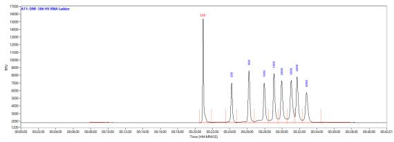
Representative HS RNA Ladder result using the Fragment Analyzer system with the DNF-472 HS RNA kit (15 nt). Method: DNF-472T33 (Total RNA analysis method, Capillary Array Short). Peaks annotated by size (nt). RFU values may differ between instruments.
