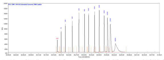
Representative HS Genomic DNA Ladder result using the Fragment Analyzer systems with the DNF-468 HS Genomic DNA 50 kb kit. The peaks are annotated by size (bp). Method: DNF-468-33 (short capillary array). RFU values may differ between instruments.
