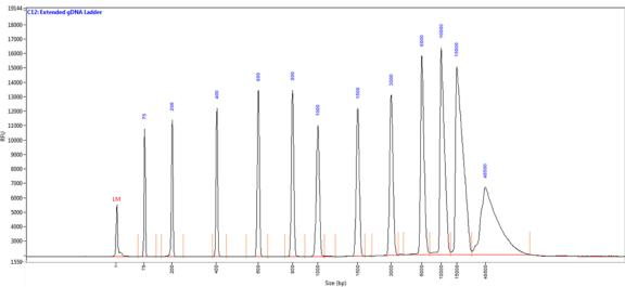
Representative Extended Genomic DNA Ladder result using the Fragment Analyzer systems with the DNF-467 Genomic DNA 50 kb kit. The peaks are annotated by size (bp). Method: DNF-467-33 (short capillary array). RFU values may differ between instruments.
