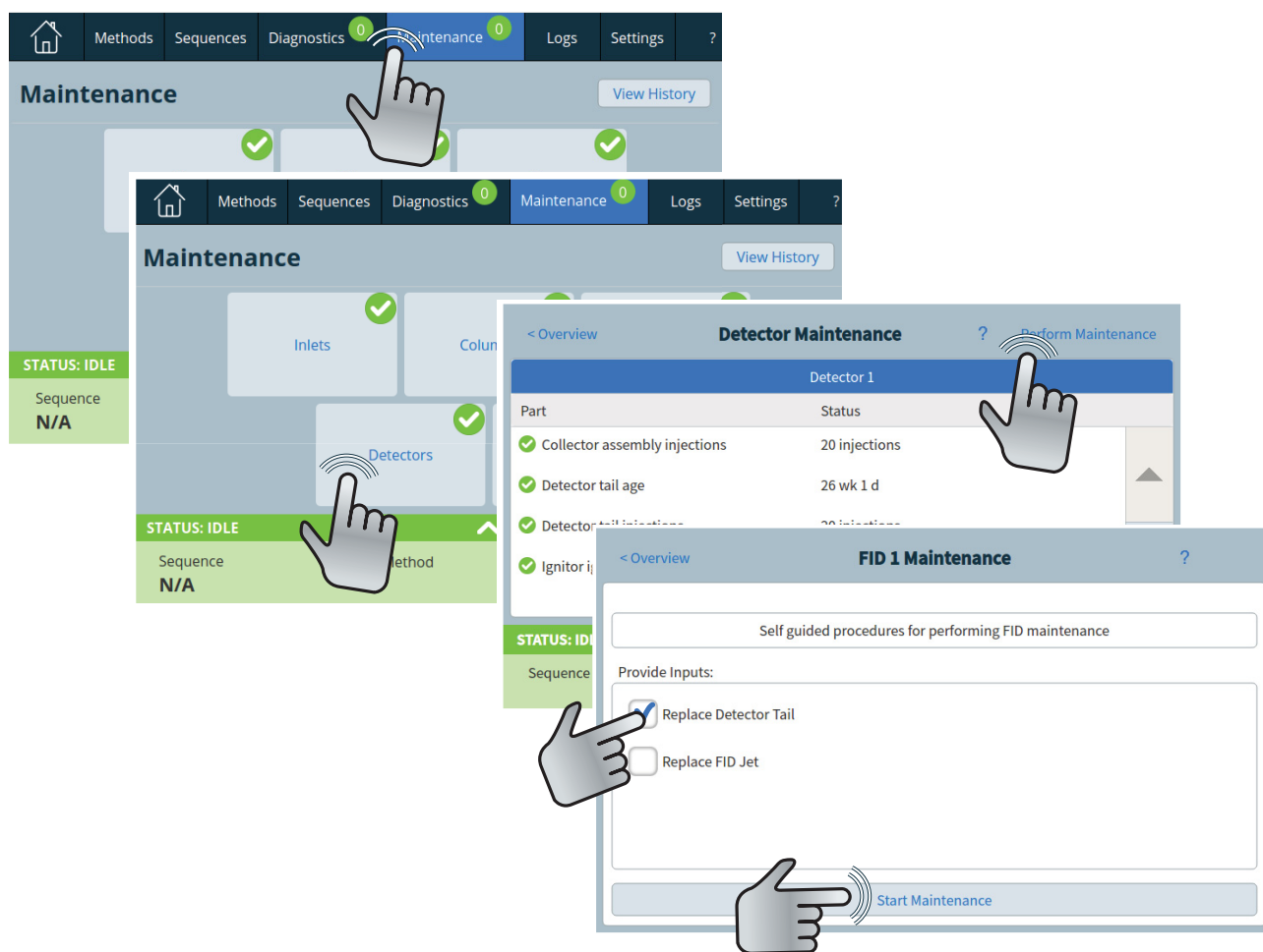
Figure 9 Launching the maintenance wizard
