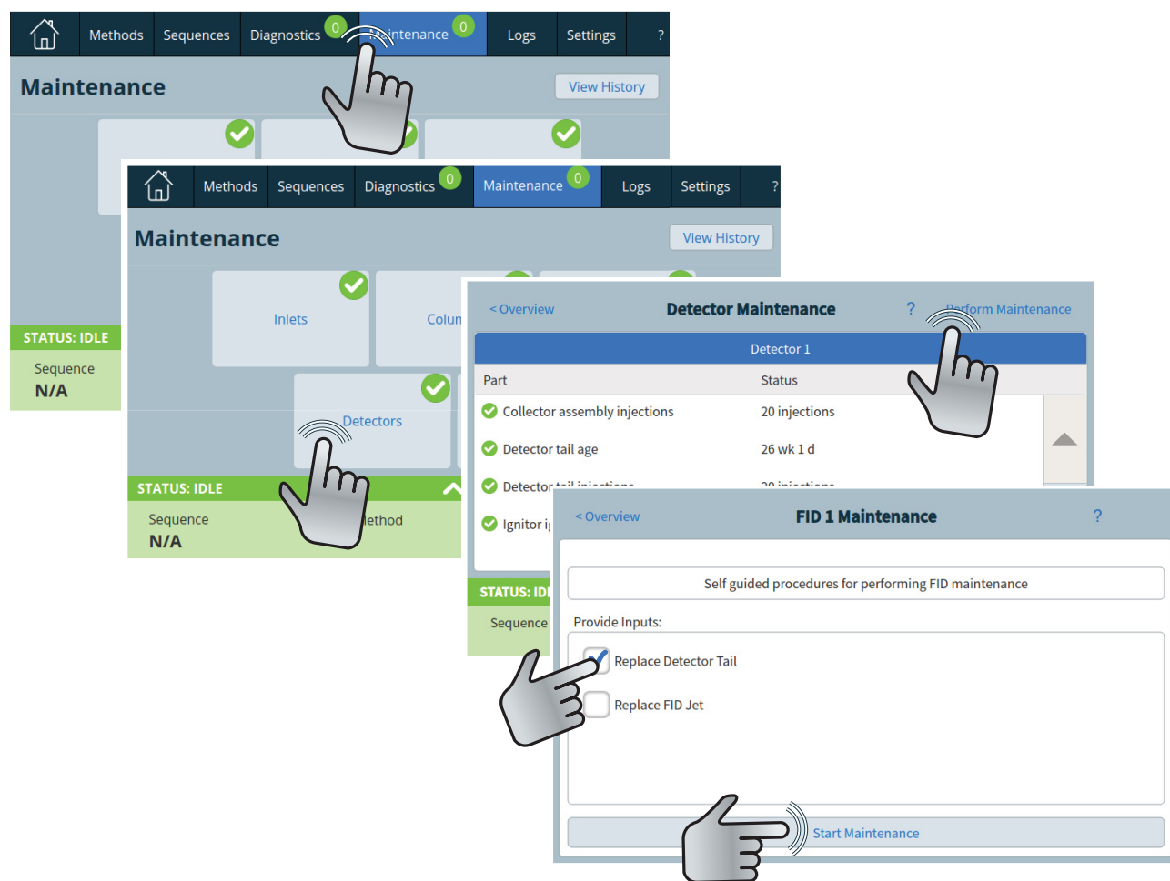
Figure 8 Launching the maintenance wizard
