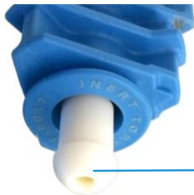
Figure 2. PTFE ball joint attached to the injector tube
