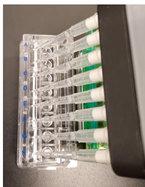
Figure 5. An eight-channel P200 pipettor is used to fill the moat on the utility plate.
