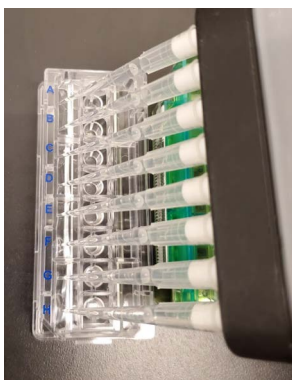
Figure 6. An eight-channel P200 pipettor is used to fill the moat on the utility plate.
