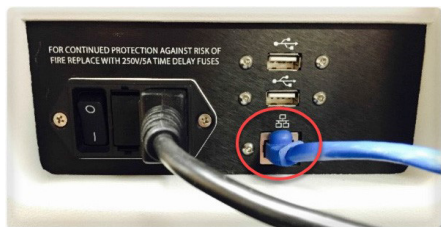
Figure 30. Ethernet port with wired network connection cable.
