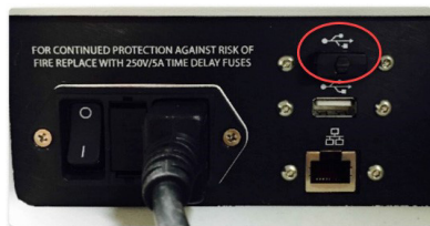
Figure 31. USB WiFi adapter inserted into an available USB port on the back of the XFp Analyzer.
