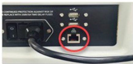
Figure 29. Ethernet (RJ-45) jack location outlined in red.
