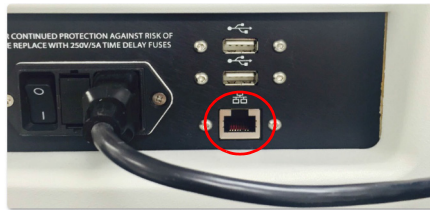
Figure 28. Ethernet (RJ-45) jack location outlined in red.
