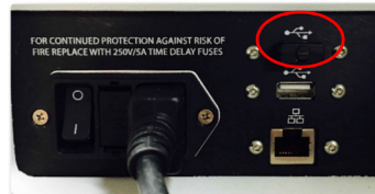
Figure 30. USB WiFi Adapter inserted into an available USB port on the back of the XFp Analyzer.
