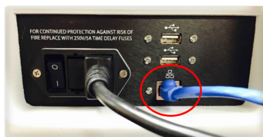
Figure 29. Wired network connection with Ethernet cable.
