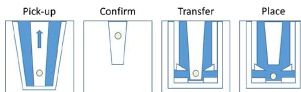
**Figure 4** Transferring spheroids
