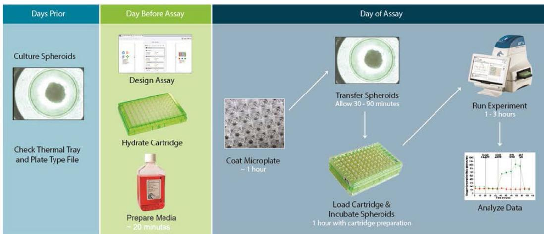
**Figure 2** Agilent Seahorse XFe96 Spheroid Microplate Assay Workflow
