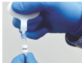
Figure 4 Removing reagent caps Hold the tube in gloved hand and roll thumb in forward motion over the cap to loosen or, using the decapping tool provided, insert the tooth of decapper into the inner lip of the cap and gently rotate the tool backwards.
