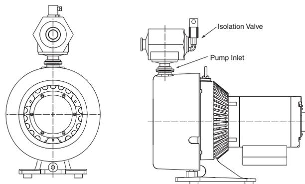
**Figure 6 Isolation Valve Location**
