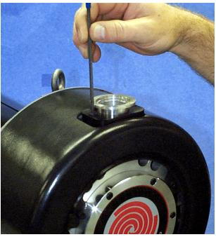
10. Secure the fitting with two M5x16 screws.
