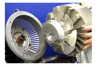
7. Remove pump module from the frame.
