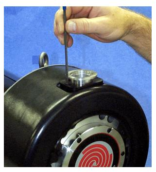
1. Remove the two M5x16 screws from the intake assembly.
