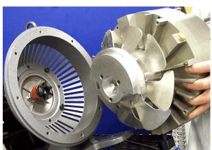
5. Install pump module on frame, aligning fingers on fan assembly with fingers on coupling. Assure proper fit of dowel pins on mating holes in frame.
