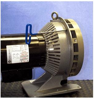
6. Remove the four M6x16 screws that attach the pump module to the frame.
