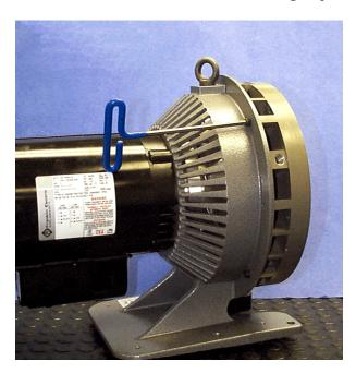
6. Secure pump module to frame with four M6x16 screws.
