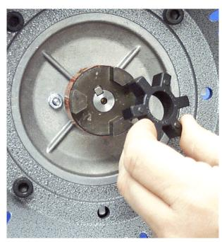
4. Insert spider in motor coupling.
