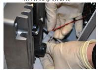
Remove 4 screws using 4 mm Thandle wrench to separate outboard housing from orbiting plate.
