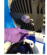
Remove 4 screws using 4 mm T-handle wrench to separate outboard housing from orbiting plate. Make sure pump is vented before attempting to separate scrolls.
