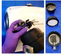
Unfasten 3 screws on front cowling using 6 mm T-handle wrench.
