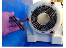
4. Remove front cowling and disconnect fan connector; set front cowling aside.
