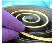
9. Apply a trace amount of grease (provided) on new O-ring and install.
