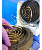
Clean both metal scrolls using abrasive scrubbing pad, low lint cloth, and low lint cleaning swabs. If a cleaning fluid is necessary or desired, use isopropyl alcohol (not included). Do not use water, detergent, or home/industrial cleaning products. Do not used compressed air or aero duster.
