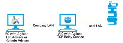
These types of setup are typical in networked laboratories where an instrument controller is installed with two network cards and applications are running on a server, but can also be used to isolate the instruments from the *company LAN* for security reasons.
