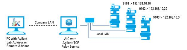
Each relay task listening to a dedicated port may start up to 10 connections. So, if Agilent Lab Advisor or Remote Advisor is started a second time from another PC, and the HPLC instrument is capable of hosting more than one connection at the same time, the relay service can serve both controllers to establish connections to the instrument.
