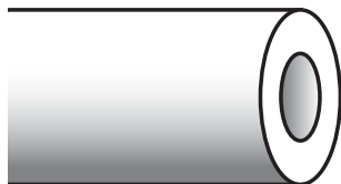
Figure 6 Properly cut tubing
