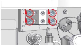
5 Connect the outlet of solvent A (upper row) to the top degasser inlet and the outlet of solvent B (lower row) to the bottom degasser inlet. Put the solvent bottles into the solvent cabinet. Connect the bottle heads of solvents A1 and A2 to the inlets in the upper row, see labels on valve assembly. Connect the bottle heads of solvents B1 and B2 to the inlets in the lower row, see labels on valve assembly.
