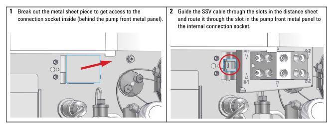
3 Carefully plug in the connector of the solvent selection valve into the internal connection socket on the left side of the slot behind the pump front metal panel.
