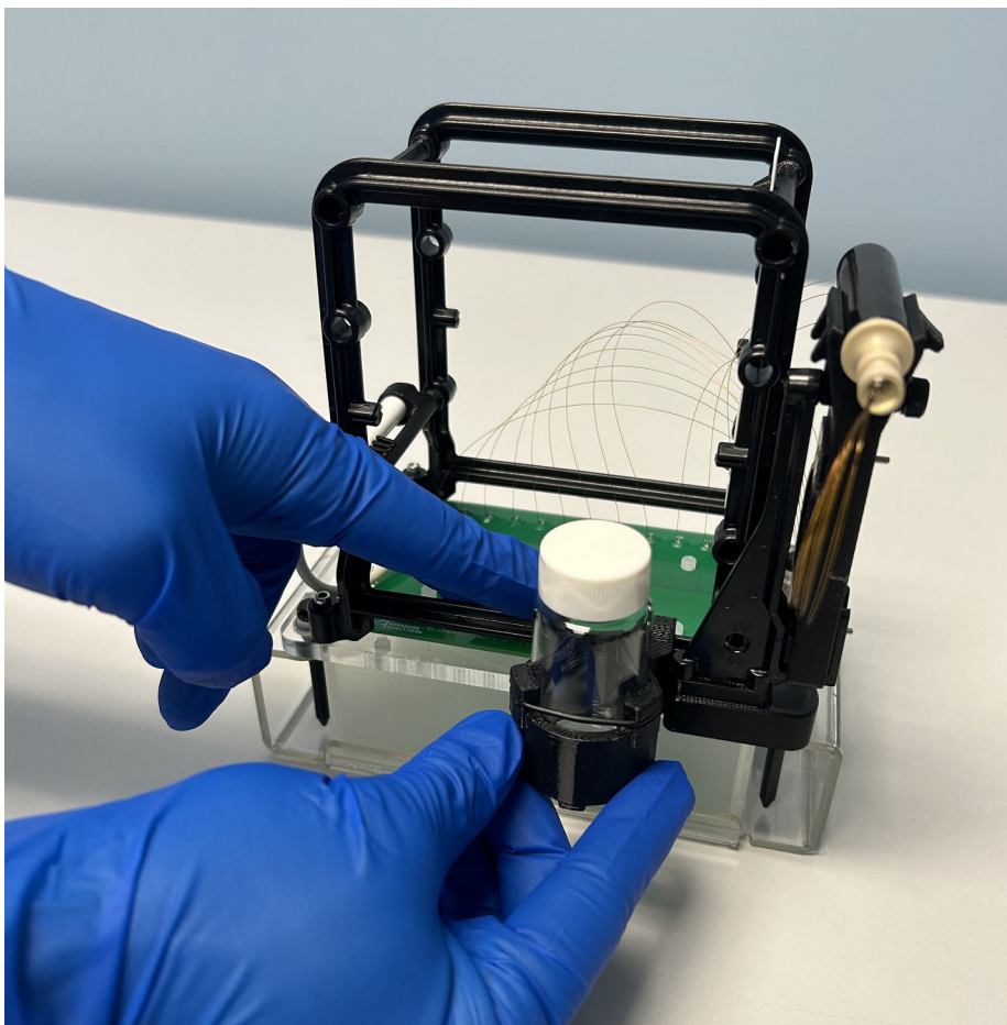
Figure 111 Array spindle storage device installation
