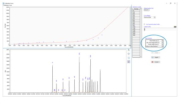
Figure 63 Calibration Curve screen showing improperly fit size calibration from Figure 62
