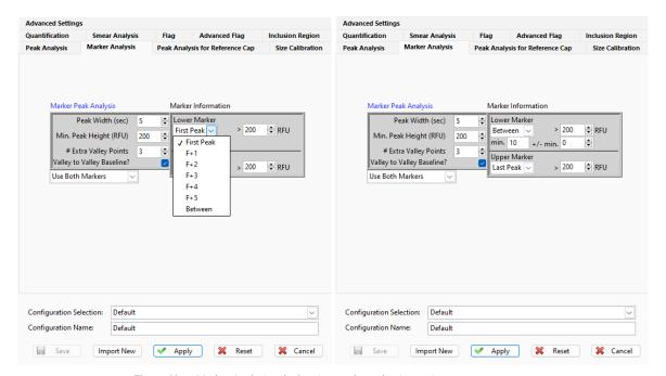
Figure 42 Marker Analysis tab showing marker selection options
