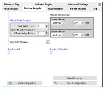
Figure 51 Marker Analysis tab in Set Individual Parameters dialog
