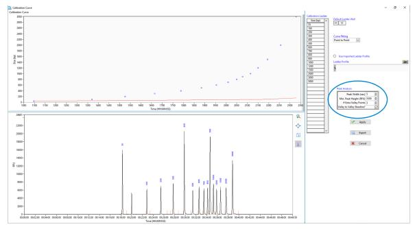
Figure 61 Calibration Curve screen showing improperly fit size calibration from Figure 60.
