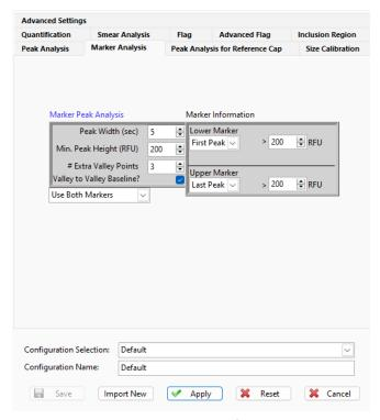
Figure 41 Marker Analysis tab in Global Configuration dialog
