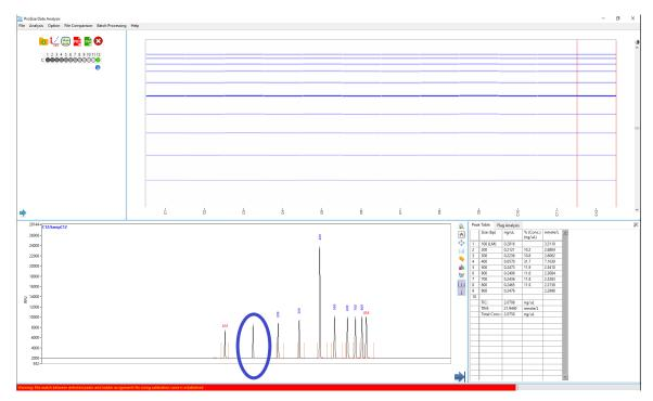
Figure 60 Main screen showing improperly fitted size calibration (not enough integrated peaks). Solution to correct: In the **Peak Analysis** table lower the Min. Peak Height (RFU) threshold to integrate missing peak (circled in blue).
