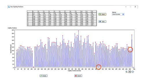
Figure 94 View Capillary Positions window where capillary is not assigned properly (circled in red)
