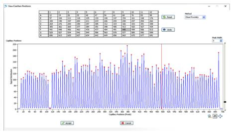
Figure 96 Manually deleting pixel 495 by selecting it, and click [Delete]
