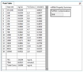
Figure 22 Peak Table form on main screen when in mRNA mode
