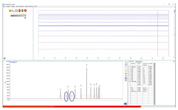
Figure 62 Main screen showing improperly fitted size calibration (too many integrated peaks, circled in blue). Solution to correct: increase the Min. Peak Height (RFU) threshold to no longer integrate extra peaks.
