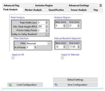
Figure 29 Peak Analysis tab in Set Individual Parameters dialog
