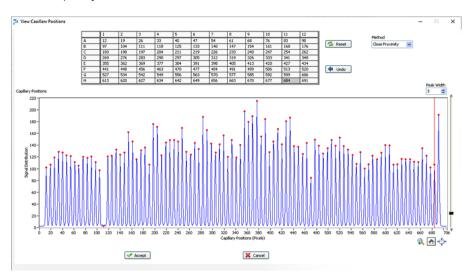
Figure 98 Alignment after clicking [Insert] at the rightmost position and using the keyboard arrow to move the vertical cursor to pixel 684. Capillary positions are now correctly located. Press **Accept** to save.
