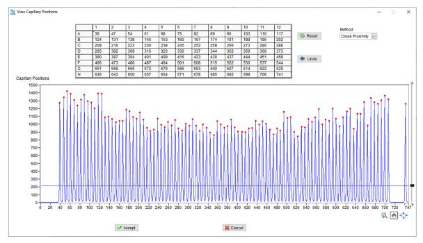
**Figure 93** Capillary Positions window after pressing **Reset**. A blue horizontal cursor can be used to select the threshold for locating capillary positions.
