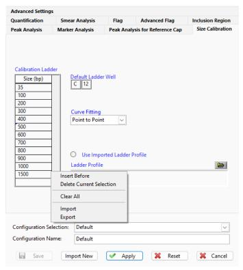
Figure 56 Size Calibration tab in the Global Configuration dialog
