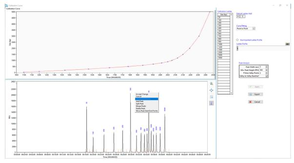
Figure 59 Figure Calibration Curve screen showing properly selected size calibration ladder
