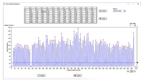
Figure 95 View Capillary Positions window showing misaligned capillary not reset by threshold
