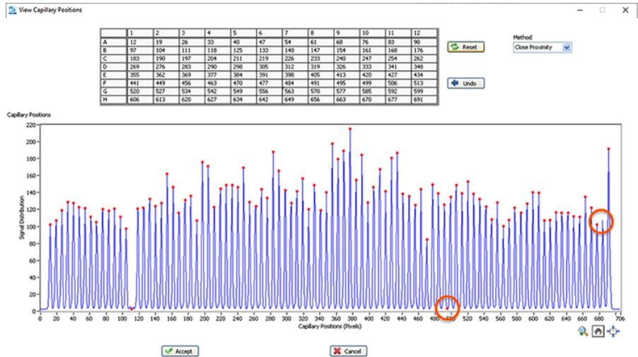
**Figure 94** View Capillary Positions window where capillary is not assigned properly (circled in red)
