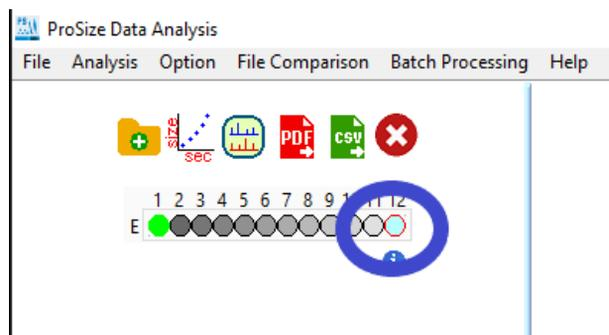
**Figure 58** Main screen: The Size Calibration well H12 is marked in blue in the Plate Map (circled in blue to highlight position of reference capillary).
