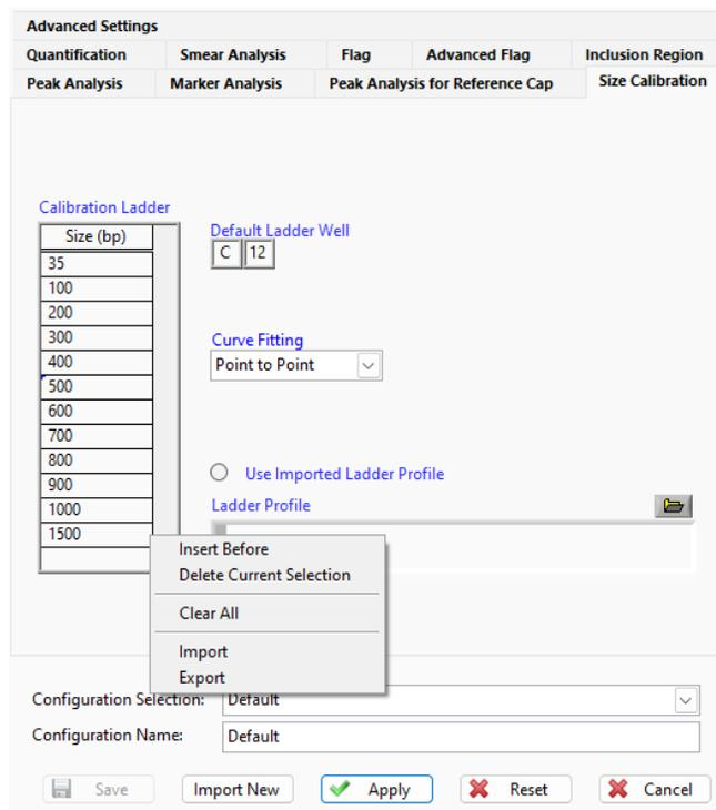
**Figure 44** Size Calibration tab in Global Configuration dialog
