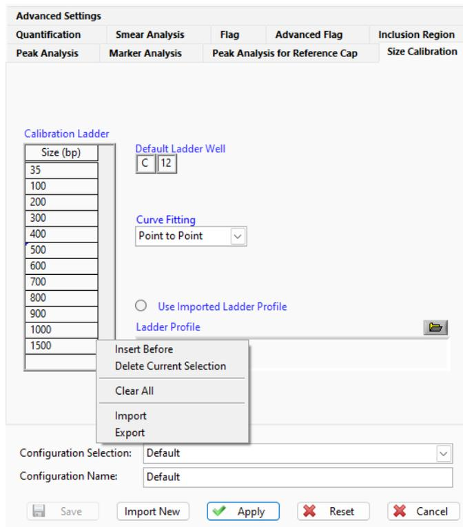
**Figure 56** Size Calibration tab in the Global Configuration dialog
