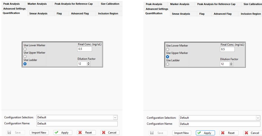
**Figure 45** Quantification tab in Global Configuration dialog (Left: **Use Ladder** selected; Right: **Use Upper Marker** selected)
