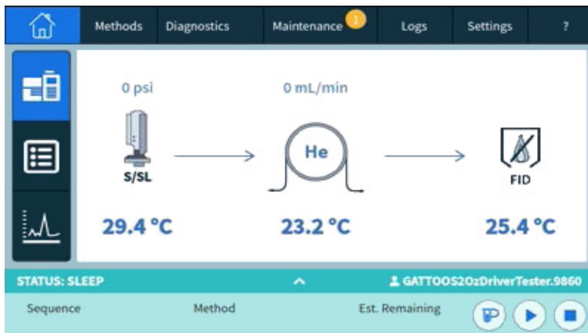
Figure 2 Intuvo local user interface (LUI) - Instrument Status
