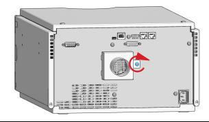
**2** Push the adapter into the grid and turn it sidewards, so that its latch covers the hole for the holding screw.
