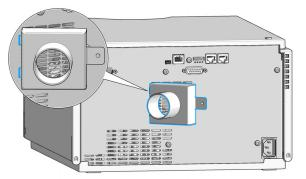
3 Use the screw delivered in the Exhaust tube adapter kit to fasten the adapter latch to the rear of the fraction collector.
