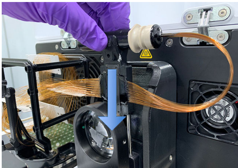
Figure 83 Instrument top compartment – array window placement
