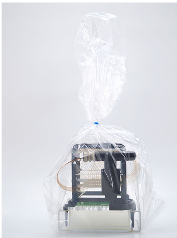
Figure 75 Capillary array shipping box – remove plastic shipping cover
