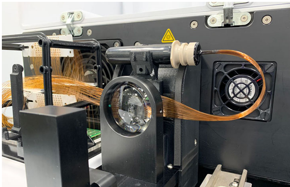
Figure 84 Instrument top compartment – capillary array bundle removal
