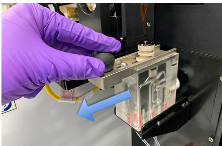
Figure 64 Instrument top compartment – capillary reservoir connector slide
