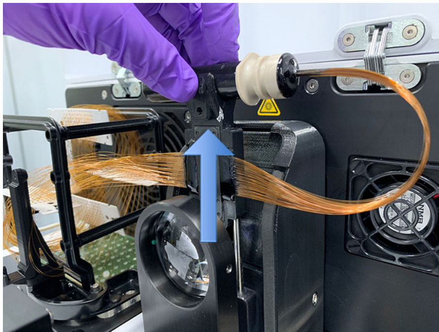
Figure 69 Instrument top compartment – remove capillary array window
