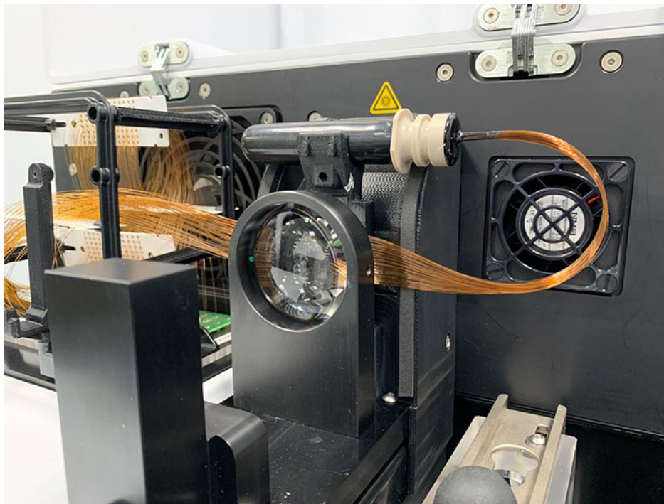
Figure 68 Instrument top compartment – storing covered capillary array bundle
