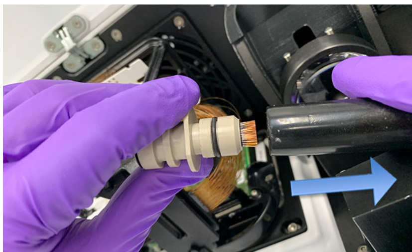
Figure 85 Instrument top compartment – removing protective cover
