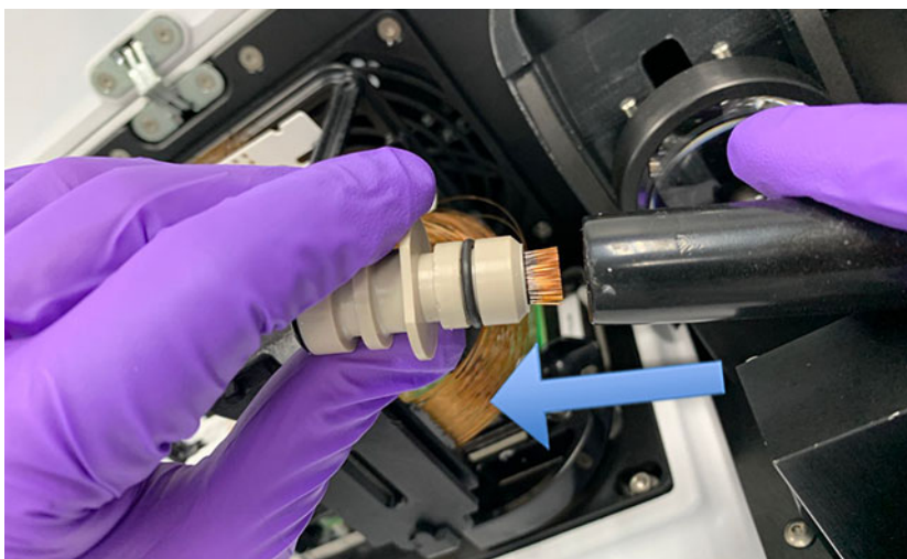
Figure 67 Instrument top compartment – installing protective cover
