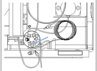
4 Install the union between the seat capillary and the other side of the seat extension loop. Store the extension loop in the leak tray.
