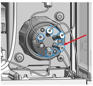
3 Install the 400 or 1400  $\mu L$  seat extension loop (longer side) to the injection valve (port 5).
