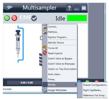
**2** In the configuration menu change seat capillary to the value of the installed extended seat capillary (400  $\mu$ L) or 1400  $\mu$ L) and press **OK**.
