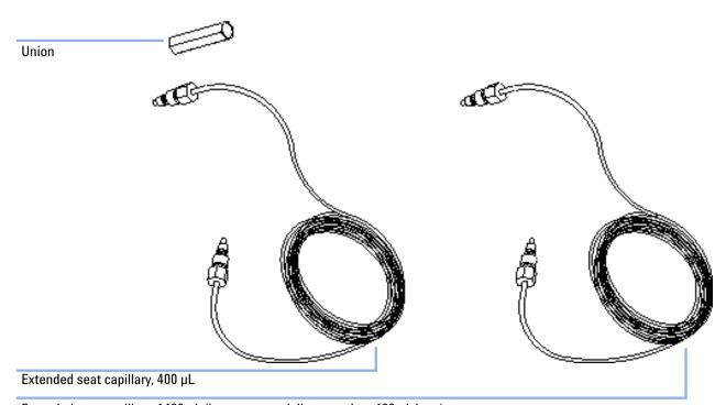
Extended seat capillary, 1400  $\mu$ L (larger external diameter than 400  $\mu$ L loop)
