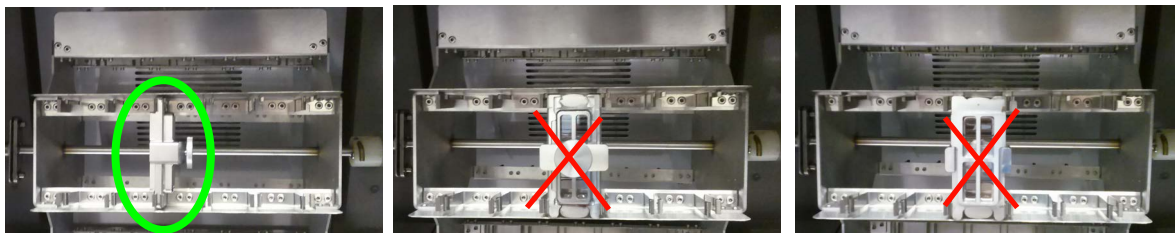
Figure 18 Assembled chambers in correct (left) and incorrect (middle and right) orientations
