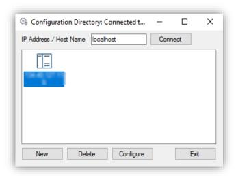
5 Selecting New opens the Agilent Configuration Editor. Highlight Agilent 1100/1200/1260/1290 LC (or Agilent 1120/1220 LC Systems) and select Auto Configure.
