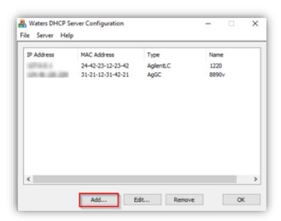
5 Enter the IP Address, MAC Address (can be arbitrary), and Serial Number or a Unique Name. Select the Instrument Type AgilentLC from the drop-down list. Confirm with OK. IP and MAC address are checked for duplicates on the same instrument controller. Once created editing existing DHCP configurations is not possible. The system must be removed and added again.
