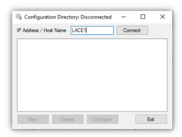
**12** When successfully connected, all configured instruments are shown for this instrument controller. Select the instrument to be deleted and click **Delete**.
