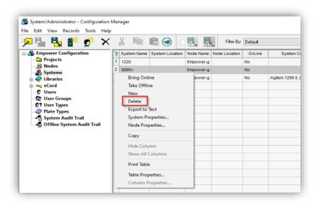
4 Confirm the deletion with **Yes** and select **Delete All** to remove the system from the node and remove it from all user accounts on this database.
