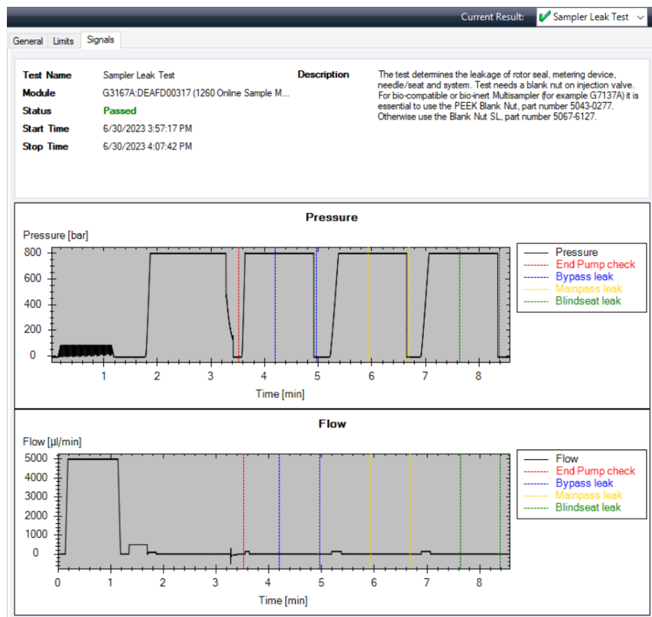
Figure 37: Sampler Leak Test passed
