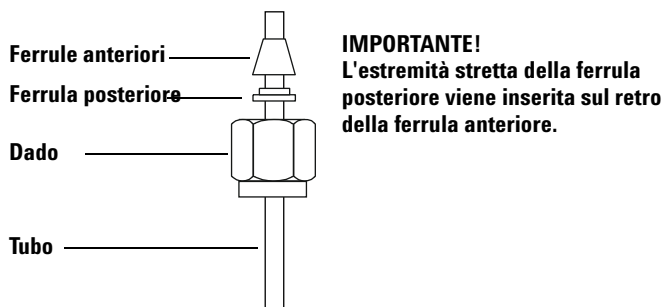
Figura 9 Dadi e ferrule Swagelok
