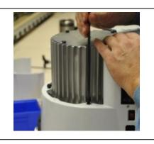
6. Loosen and remove the two M6x16 mm bolts on the bottom of the base to the pump module using a 5mm hex key. Move the base assembly up enough to facilitate removal of the Rubber Thermal Protector.
