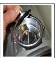
9. Remove the O-ring from the assembly and discard. Remove the 10-32 threaded orifice and discard.
