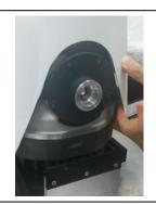
7. Remove the thermal rubber protector from the inlet assembly and discard.
