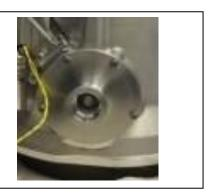
8. Loosen the four M4x10mm screws holding the inlet flange on to the frame. Remove the inlet flange from the top of the frame assembly. Remove the VPI spring and diaphragm/piston from the frame assembly. Discard the piston assembly.
