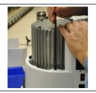
15. Reinstall the rear cowling on to the pump assembly.
