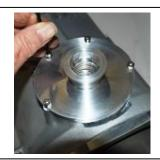
13. Install a new Thermal Rubber Protector onto the inlet assembly.
