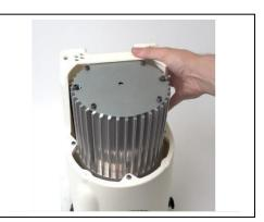
5. Loosen the three M6x20mm that secure the top part of the base to the Pump Head.
