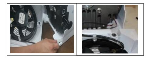
18. Attach the front cowling to the pump using three M8x20mm flange bolts. Tighten with 6mm Hex Key. Torque screws to 11.3 Nm if a torque wrench is available.
