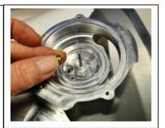
10. Install a new 10-32 threaded orifice. Apply LVP grease to a new O-ring and install it into the O-ring groove.
