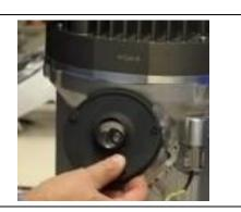
14. Reseat the base assembly. Verify that all connections are in place and that there are no pinched wires. Tighten the five screws that hold the base assembly in place.
