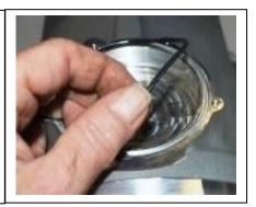
11. Install a new O-ring from the kit into the diaphragm/piston assembly. Install the new diaphragm/piston assembly from the kit into the frame. Install the spring onto the diaphragm/piston assembly.
