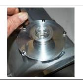
18. Install a new Thermal Rubber Protector onto the inlet assembly.
