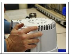
21. Install the six self-tapping screws and two washers that hold the rear cowling to the chassis and front cowling.
