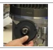
19. Reseat the base assembly. Verify that all connections are in place and that there are no pinched wires. Tighten the five screws that hold the base assembly in place.
