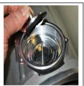
9. Remove the O-ring from the assembly and discard. Remove the 10-32 threaded orifice and discard.
