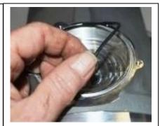
16. Install the new diaphragm/piston assembly from the kit. Install the spring onto the diaphragm/piston assembly.
