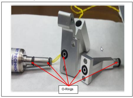
13. Reassemble the new solenoid into the mounting fixtures.
