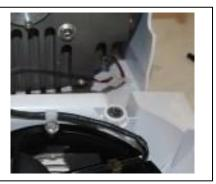
23. Attach the front cowling to the pump using three M8x20mm flange bolts. Tighten with 6mm Hex Key. Torque screws to 11.3 Nm if a torque wrench is available.
