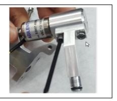
14. Mount the solenoid onto the pump frame. Secure to the frame using two M4 screws.
