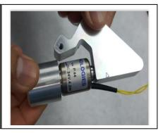
12. Replace the solenoid with the one included in the kit. Remove and replace the five O-rings in the assembly with the new O-Rings included with the kit.
