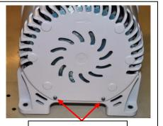
Tighten rear cowling screws and washers.
