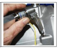
11. Remove the solenoid from the mounting brackets.
