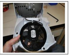
3. Disassemble the rear cowling by remove the six self-tapping screws and two washers that hold the rear cowling to the chassis and front cowling using a Philips head screwdriver.
