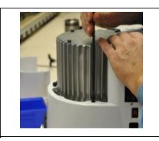
6. Loosen and remove the two M6x16 mm bolts on the bottom of the base to the pump module using a 5mm hex key. Move the base assembly up enough to facilitate removal of the Rubber Thermal Protector.
