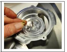
10. Remove the solenoid assembly from the frame by removing the two M4 screws.
