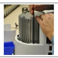
20. Reinstall the rear cowling on to the pump assembly.
