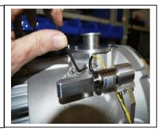
15. Install a new 10-32 threaded orifice. Apply LVP grease to a new O-ring and install it into the O-ring groove.
