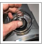
17. Install the new Inlet Flange assembly into the frame assembly and secure with four M4x10 mm screws.
