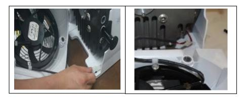
15. Attach the front cowling to the pump using three M8x20mm flange bolts. Tighten with 6mm Hex Key. Torque screws to 11.3 Nm if a torque wrench is available.
