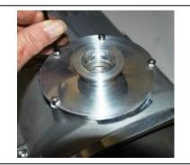
10. Install a new Thermal Rubber Protector onto the inlet assembly.
