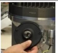
11. Reseat the base assembly. Verify that all connections are in place and that there are no pinched wires. Tighten the five screws that hold the base assembly in place.
