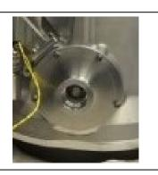
8. Loosen the four M4x10mm screws holding the inlet flange on to the frame. Remove the inlet flange from the top of the frame assembly. Remove the VPI spring and diaphragm from the frame assembly. Remove the O-ring from the assembly and discard.
