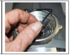
9. Apply LVP grease and install a new O-Ring into the groove. Install the VPI spring and diaphragm into the frame assembly. Using a 3mm allen wrench, install the four M4x10mm screws holding the inlet flange on to the frame. Torque to 1.6 N.m if a torque wrench is available.
