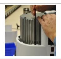
12. Reinstall the rear cowling on to the pump assembly.
