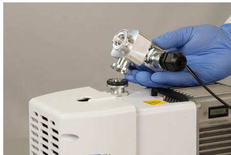
Figure 29 Mount Inlet Valve with IDP-4 Pump
