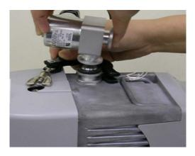
Figure 10 Mount Inlet Valve with IDP-3 Pump
