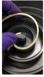
Apply a trace amount of grease (provided) on O-ring. Install new O-ring.
