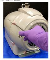
Remove front cowling and disconnect fan connector; set front cowling aside.
