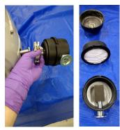
Unfasten 6 screws on front cowling using 4 mm T-handle wrench.
