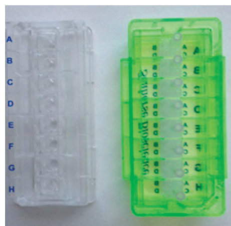
Figure 2. Utility plate (left) next to upside down sensor cartridge (right).
