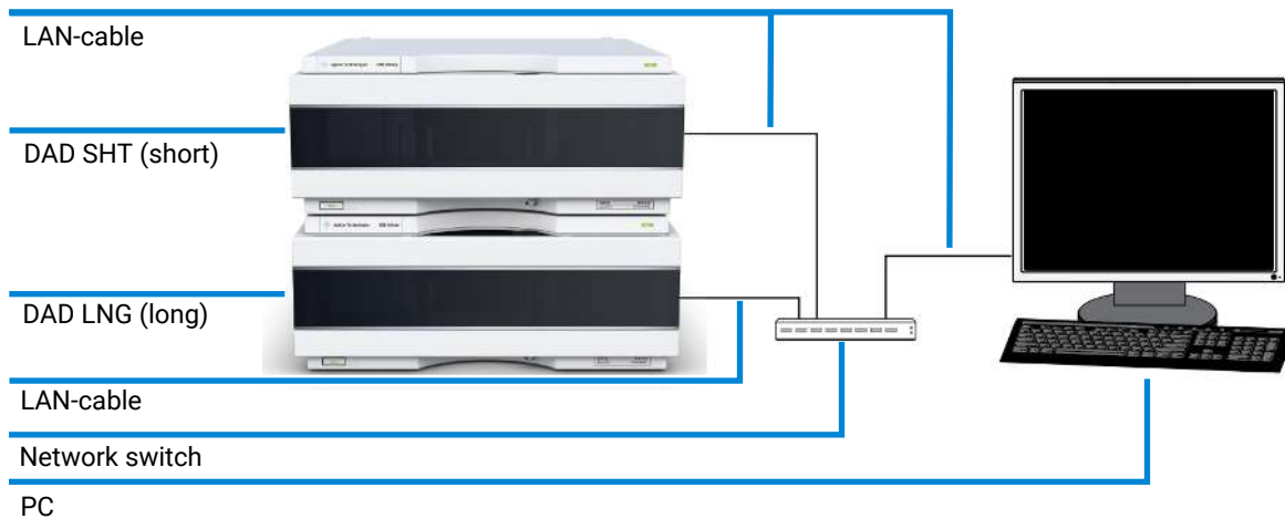
Figure 4: Local LAN connection to a PC (not via corporate LAN)
