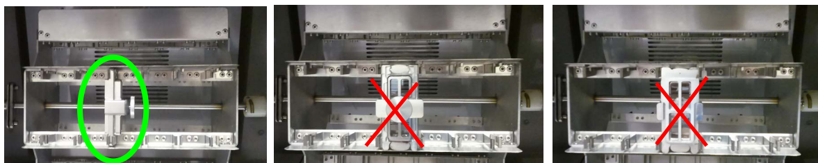
Figure 15. Assembled chambers in correct (left) and incorrect (middle and right) orientations
