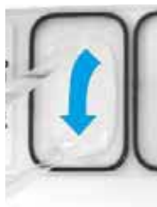
Figure 8. Drag and dispense method – Start dispensing when the pipette tip is near the top of the well. Finish dispensing when the pipette tip is near the bottom of the well.
