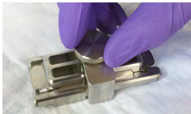
Figure 12. Tightening of the thumbscrew on the clamp
