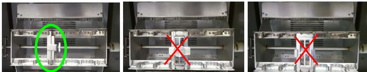
Figure 13. Assembled chambers in correct (left) and incorrect (middle and right) orientations
