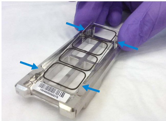
Figure 4. Chamber base, guide posts denoted with arrows
