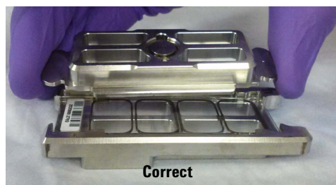
Figure 8. Chamber cover in correct (left) and incorrect (right) orientations
