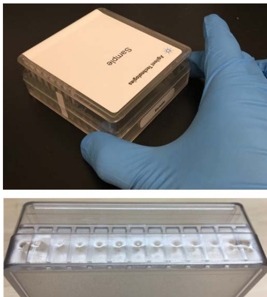
Figure 19. Gripping the base at the indentations (top) and close-up of the indentations (bottom)
