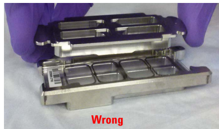
Figure 8. Chamber cover in correct (left) and incorrect (right) orientations
