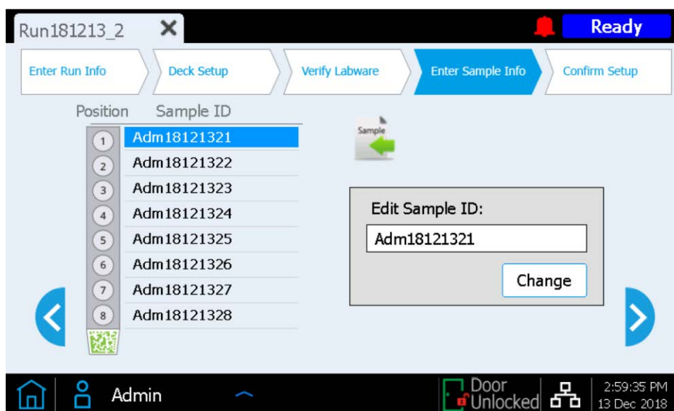
Figure 4 Magnis touchscreen interface used for manual sample assignment during a run.
