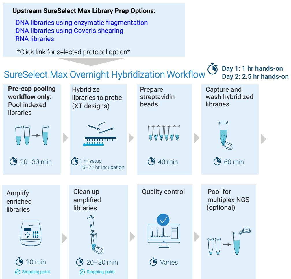
Figure 1 Summary of the SureSelect Max Overnight Hyb target enrichment workflow segment, including optional stopping points and estimated time requirements. Estimates are guidelines for 16 reaction runs. Timing for runs using different protocol parameters may vary.
