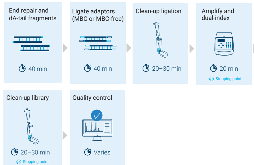
Figure 1 Summary of the SureSelect Max mRNA library preparation workflow, including optional stopping points and estimated time requirements. Estimates are guidelines for 16 reaction runs using 1000 ng input RNA. Timing for runs using different protocol parameters may vary.
