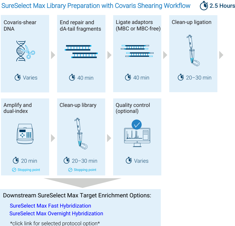
Figure 1 Summary of the SureSelect Max DNA library preparation workflow using mechanical shearing for downstream target enrichment. The estimated time requirements and optional stopping points are provided in this diagram for reference. Estimates are guidelines for 16 reaction runs using 200 ng high-quality input DNA, starting after DNA shearing. Timing for runs using different parameters may vary.
