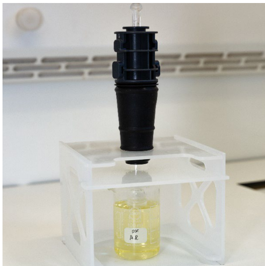
Figure 15A. Soak the torch in the aqua regia solution. Ensure the injector is immersed in the solution.
