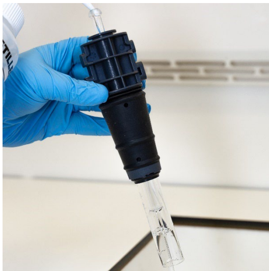
Figure 16A. Rinse the injector with deionized water through the ball joint connector.
