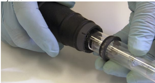
Figure 6. Torch inserted into torch body
