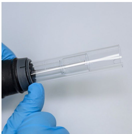
Figure 9. Removing the top seal on a semi-demountable torch by prodding it using a thumb nail
