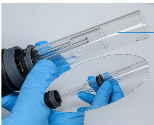
Figure 11. Removing the quartz tube-set from the torch body
