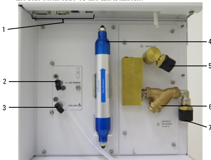
Figure 2. Input and output connections on the side of the ICP-OES instrument
