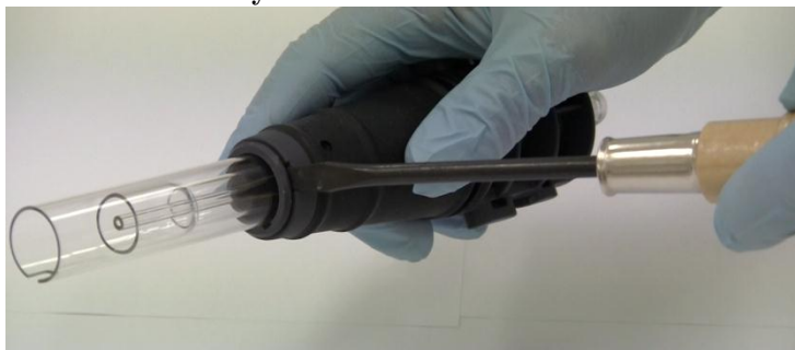
Figure 9. Separating the torch securing ring from the torch body
