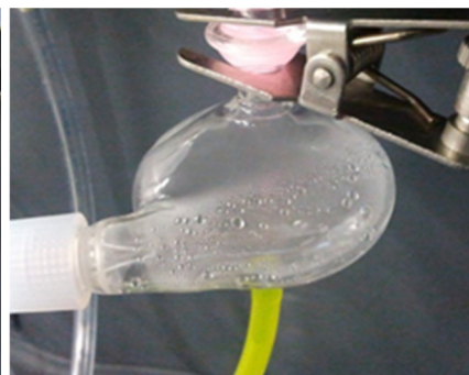
Figure 7. Incorrectly ‘wetting’ spray chamber showing droplets
