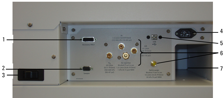
Figure 2. Input and output connections on the side of the MP-AES instrument
