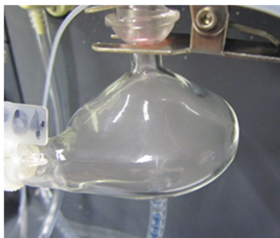
Figure 6. Correctly ‘wetting’ spray chamber with a uniform coverage
